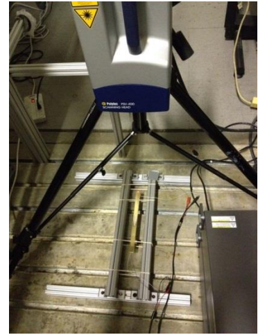
Figure 4 Experimental setup to study the traveling waves generated on a free-free beam
